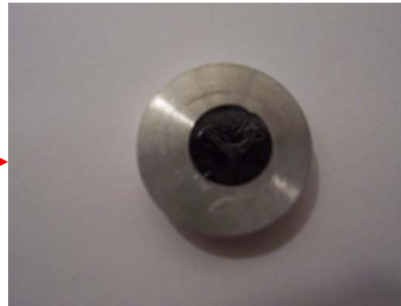
Filter coated with a 1-nm thick platinum
